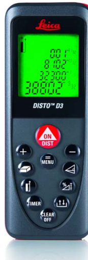
Leica DISTO™ D3 Range: 0.05m - 100m. Power Range Technology™. Accuracy: ±1.0mm. Integrated tilt sensor. Multifunctional end piece. Addition, subtraction, area, volume, min/max function. Indirect measurement, Solid angle calculation. Automatic keypad and 4-lines display illumination. Robust: IP 54 protected.
